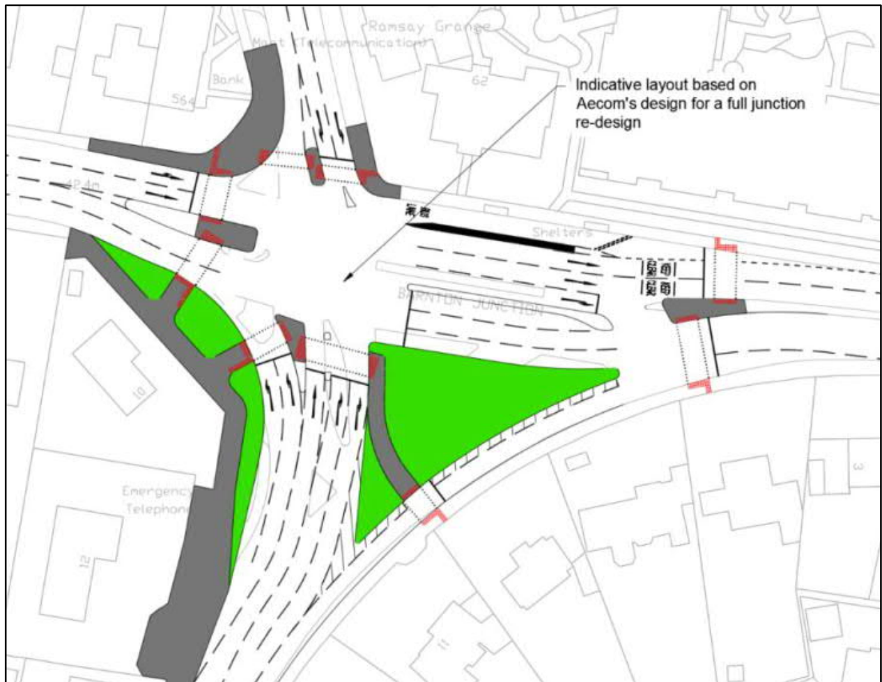
Figure 3: Option 7.1.B Proposed junction layout based on the preferred design within the Maybury Road Transport Feasibility Study, 08/05/2020
