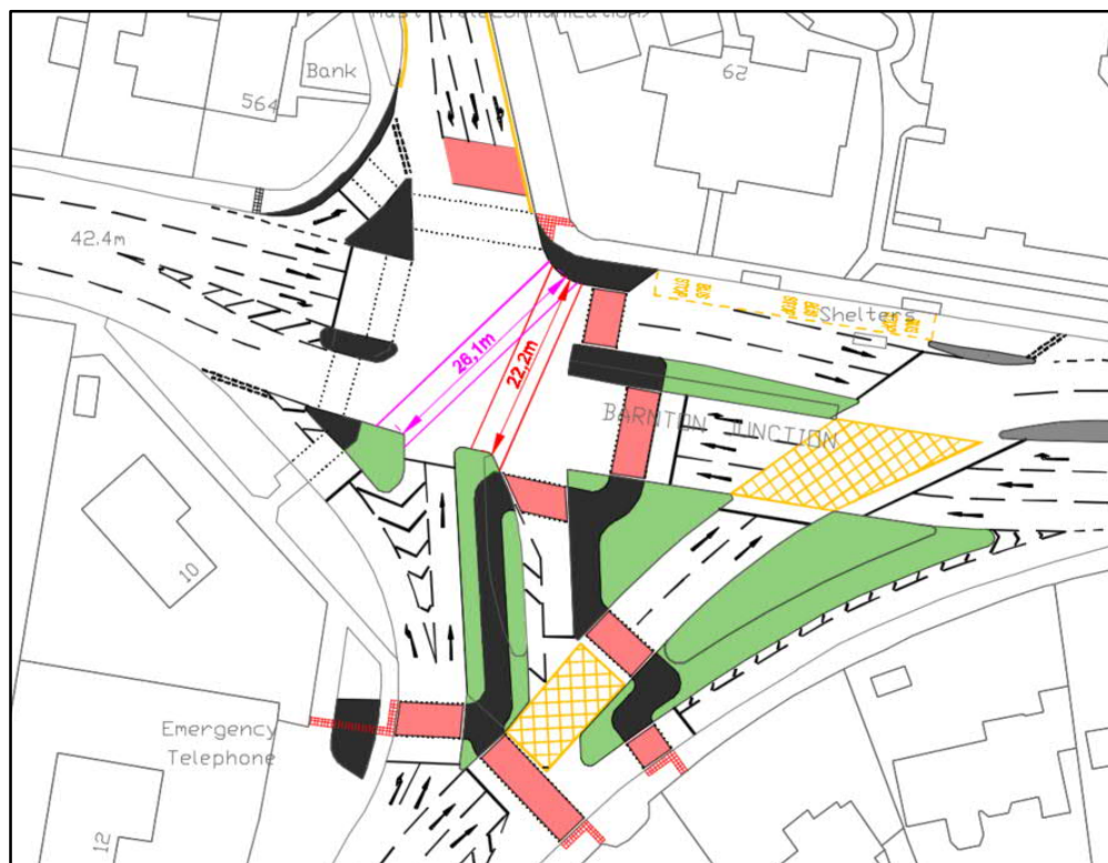
Figure 9: Possible diagonal crossings for NMUs
