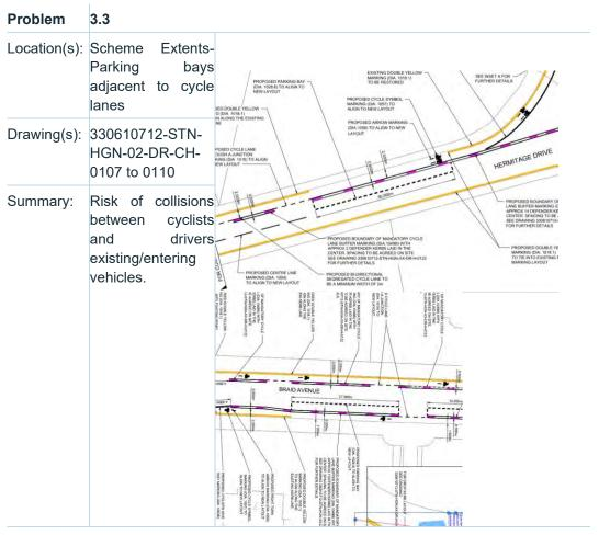
Parking bays are proposed adjacent to cycle lanes at various locations throughout the scheme extents. At these locations a 0.535m 'buffer' is proposed consisting of an 150mm road marking, 235mm kerb defender and 150mm cycle lane marking.
