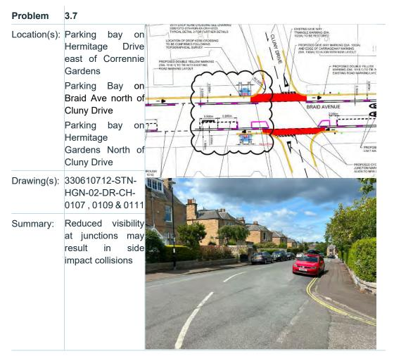
Parking bays are proposed adjacent to side road junctions at the locations noted above. When occupied, visibility to/from the junction may be obstructed which may contribute to side impact type collisions as vehicles emerge from side roads. The risk is exacerbated on Braid Avenue as parking bays have been relocated further into the carriageway from the existing kerbline to accommodate the proposed cycle lane, reducing visibility further.
