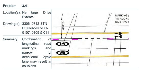
Whilst it is acknowledged a response has been provided to the potential risk due to narrow cycle lanes and proximity to kerb lines (RSA Stage 1 Problem Ref 3.2), there is a potential risk that due to the provision of double yellow lines within the narrow bi-directional cycle lane:
